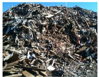
pile could then be the first material processing once this is initiated in early 2012. Regardless of the level of contamination and water damage, it is still somewhat unlikely that this supply of waste plasterboard for recycling will produce a high quality end product for use by HCL. The appearance of the rubble currently at BRRP certainly does not give rise to strong hope in this regard.
