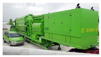
A newer version of the unit, known as the XL, can handle even higher volumes, and while somewhat larger, is still able to be transported without special permits on European and US roads. All units, powered by their own diesel generator, are fully automated, create "almost no dust" and are "almost noiseless" in operation. The output is considered very high quality with very low paper contamination in the recycled gypsum.
